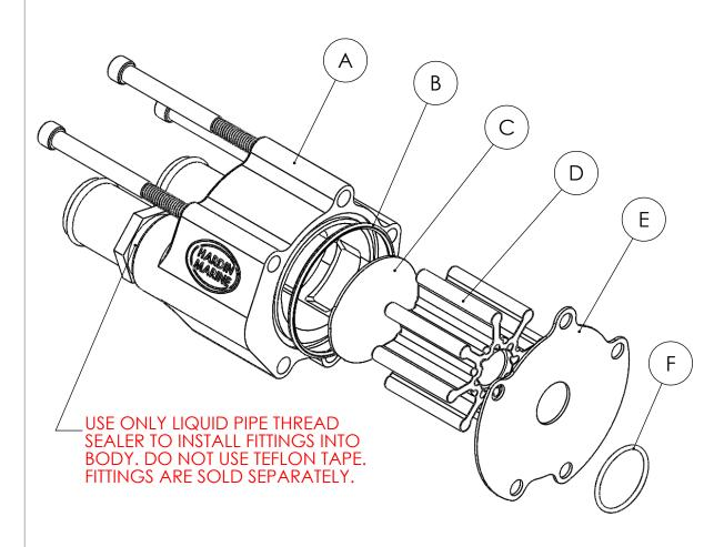
IINSTALLATION INSTRUCTIONS : 1) INSTALL WEAR PLATE (C)INTO BODY (A). 2) APPLY GREASE INSIDE BORE AREA. INSERT IMPELLER (D) INTO BORE. MAKE SURE IMPELLER BLADES ARE BENT IN THE DIRECTION SEA PUMP WILL BE SPINNING. THE BACK SIDE OF BODY SHOWS STANDARD LEFT HAND ROTATION. 3) INSTALL LARGER O-RING (B) IN THE O-RING GROOVE IN BODY. APPLY A LIGHT COAT OF GREASE TO O-RING. THIS WILL HOLD O-RING IN PLACE.
